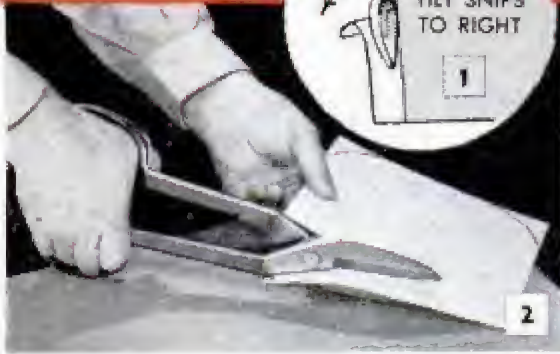
Snips should be held square with work, except aviation type which cut best with right tilt. Below, vise mounting aids in cutting thick stock
